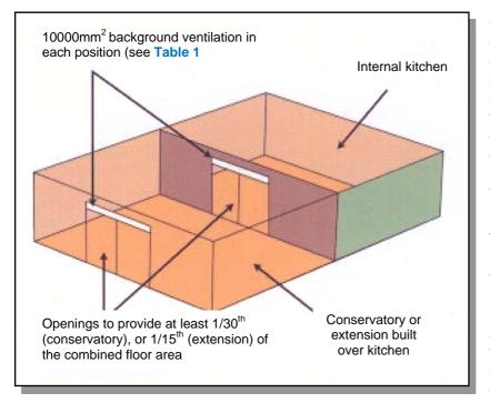
Clause 3.14.7 explains that a conservatory may be constructed over a ventilator serving a room in a dwelling provided that the ventilation of the conservatory is to the outside air and has an opening area of at least 1/30th of the total combined floor area of the now internal room and the conservatory.
